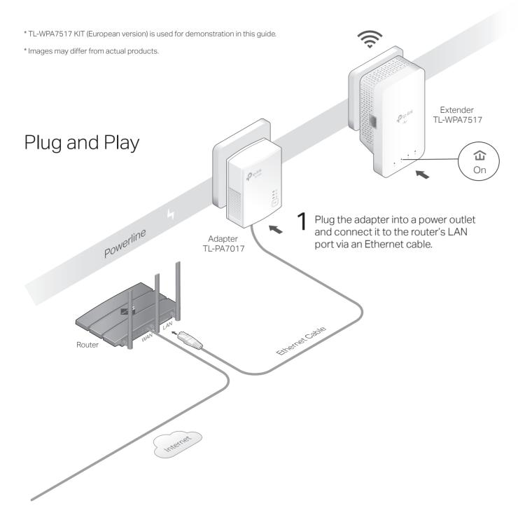
Plug the extender into a power outlet on the same electrical circuit. Wait until the extender's Powerline LED turns on.
